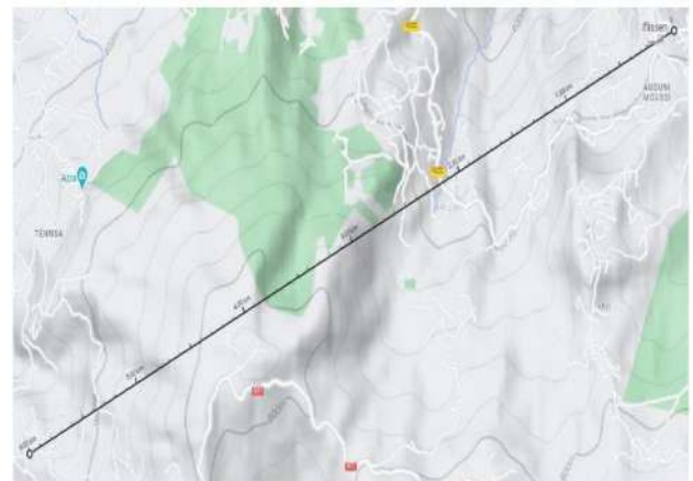
Figure 6. Map illustrates data transmission over a distance of 6 km with a clear LOS between Iflissen and Azra.
