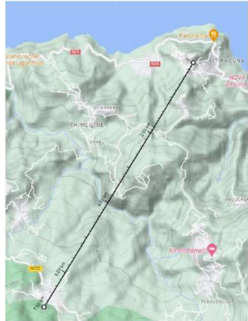
Figure 5. Map illustrates data transmission over a distance of 7 km with a clear LOS.
