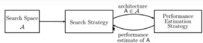
Fig. 4. Different Neural architecture search components
