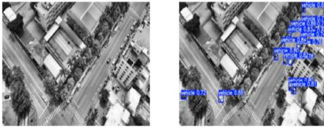
Fig.3. Vehicle detection using yolov8.
