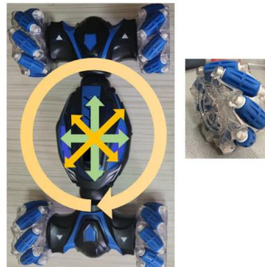
Fig. 4: Mecanum Wheeled mobile robot
