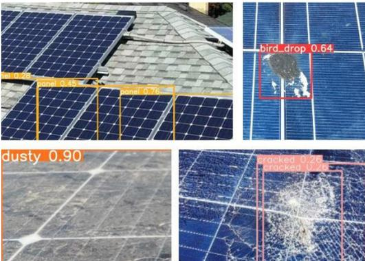
Fig. 5. YOLOv10s Detection Results
