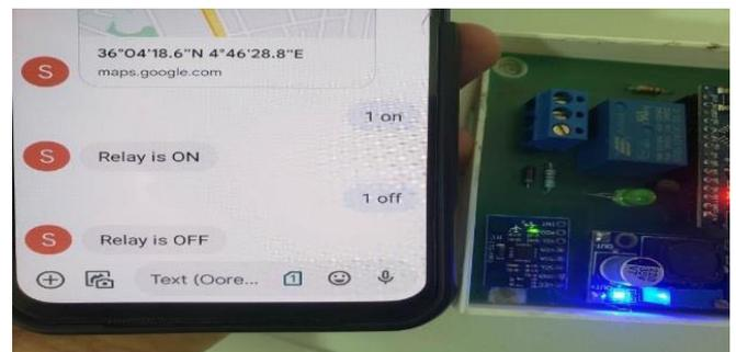
(b) Relay turning OFF-SMS 1 OFF
