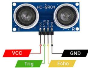
Fig5. Ultrasonic sensor
