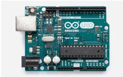
Fig1. Arduino Uno R3 board
