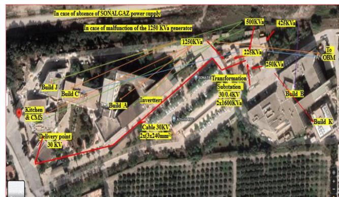
Fig. 1 Operating of the five backup power generators within TRC [2].
