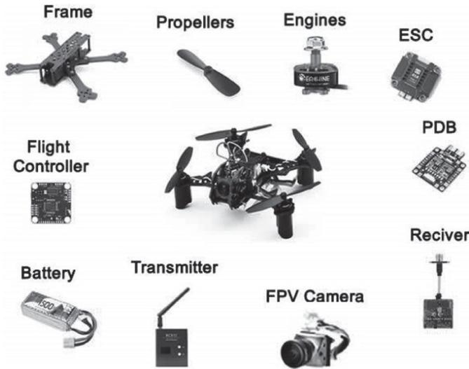
Fig. 2. Main components of UAV
