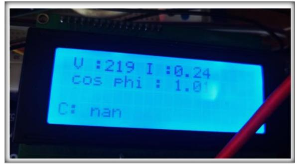
Fig. 10. Electrical characteristics of load after correction
