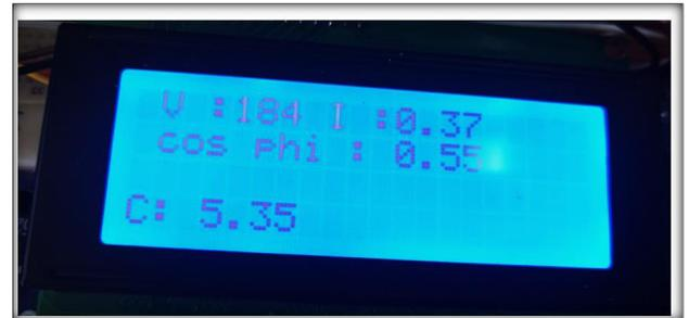
Fig. 7. Electrical characteristics of load before correction
