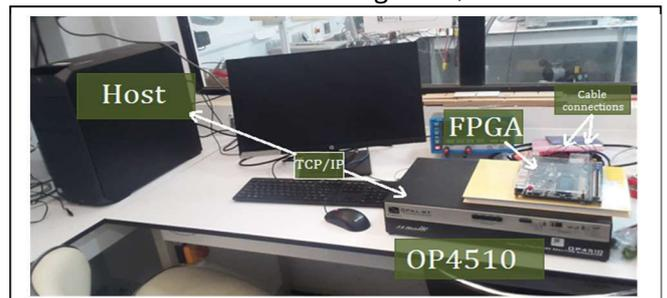
Fig. VI-1 The Final Hardware Setup of the experiment
