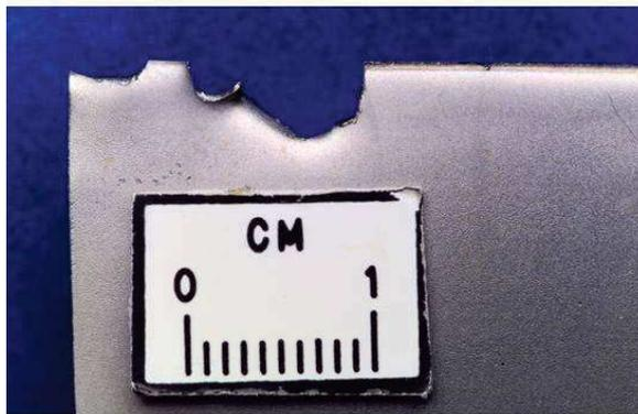
Fig. 7. Pumping Damage to a blade .
