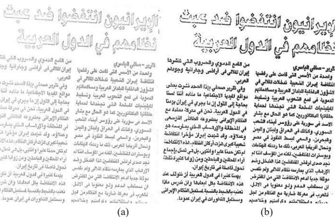
Fig. 3. Binarized document image: (a) Original image, (b) Binarized image using Sauvola thresholding.
