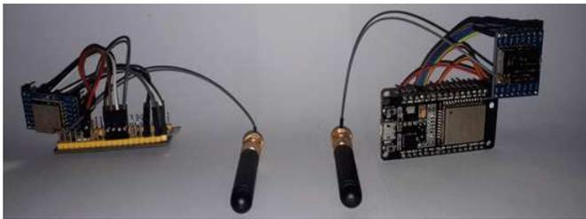
Fig. 7. End-node (left) to gateway (right) communication test (close-range).
